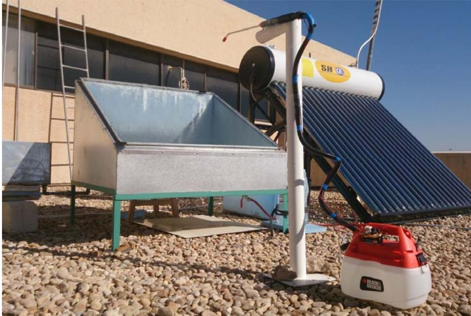
Solar Water Desalination by Evaporative Cooling
